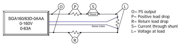
Set Power Supply output at 80V at no load, fix setting and then disable the unit. (Voltage setting was not changed for the remainder of the tests). Perform the three test series below to quantify the regulation response when high load line drop is experienced while utilizing remote sensing at the load.
